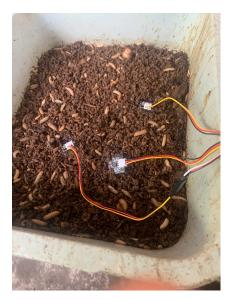
The unfortunate finding was that the cheap soil-probes won't work in the coarser medium consisting of waste food and black-soldier-fly larva.
