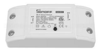
This is a big deal. The Sonoff switch can be inserted into a power-line, of a fan or a pump or something. Technically that is easy to do, but since its handling 240V it is hard to safely cut corners. The Sonoff's are ~USD4.50 and once reprogrammed to sit in the Frugal-IoT platform enable simple automated control, at around USD10, for example for a fan that comes on at high temperatures, or can be controlled remotely.
